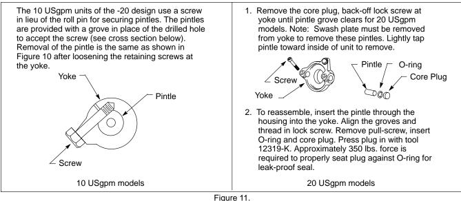
6. Yoke Removal – Figures 10 and 11 illustrate the procedure for removal of the yoke from a variable displacement unit. Yokes of the smaller units are similar in design to the larger units. Only the methods of retaining are different.
