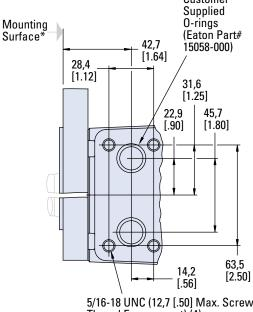
5/16-18 UNC (12,7 [.50] Max. Screw Thread Engagement) (4) or M8 x 1,25 (12,7 [.50] Max. Screw Thread Engagement) (4)
