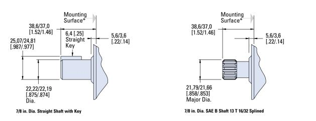
\*2 Bolt SAE B mounting flange has a greater pilot thickness and a thinner mounting plate (and of shaft to flange, add 3,3 [.13]).
