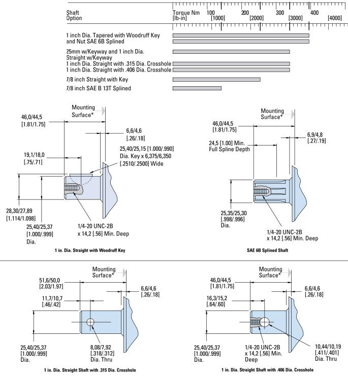
\*2 Bolt SAE B mounting flange has a greater pilot thickness and a thinner mounting plate (and of shaft to flange, add 3,3 [.13]).
