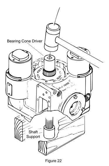
**78** Turn the pump over so the shaft is vertical and the mounting flange is down.
