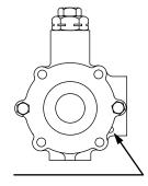
Clockwise rotation: bead on spacer and bead on pump body not aligned.
