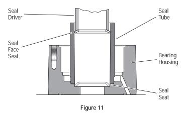
21 Place bearing housing on smooth flat surface with largest open end of housing up. Apply petroleum jelly to shaft face seal. Install seal in seal seat. Seat seal properly in groove (see Figure 11). A damaged or improperly installed shaft face seal could cause internal lubrication loss and subsequent parts wear.
