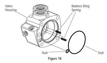
**40** Apply a light film of petroleum jelly on 8,9 mm [.35 inch] I.D. seal. Install seal in case drain groove of valve housing.
