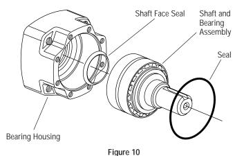
**18** Remove shaft and bearing assembly. You may need a press to remove shaft and bearing assembly (see Figure 10).
