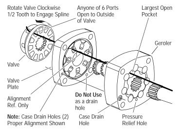
Figure 16 Timing Alignment
