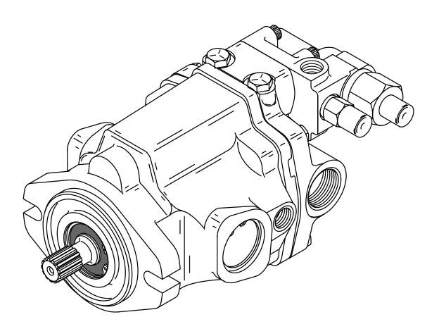
Model 70122, 0 -19 cm<sup>3</sup>/r [0-1.16 in<sup>3</sup>/r] Displacement Pressure or Pressure-Flow Compensated Piston Pumps
