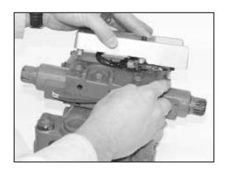
Carefully position the EP Control electronic module. Tuck all cables under the module. **Caution:** Avoid pinching cables at mounting points.
