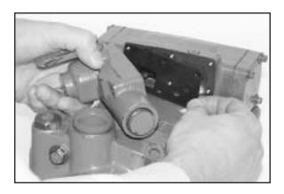
Remove the control valve gasket from the pump housing and discard.
