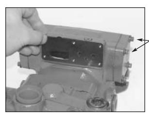
Remove top hex head cap screws on each side.
